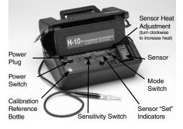
Remove the sticky-label disc from the cap of the CALIBRATION REFERENCE bottle. This disc can be reused to help seal the vial when the leak detector is not in use, or it can be discarded. DO NOT attempt to unscrew the cap, you may damage the bottle! It is filled with enough refrigerant to last approximately six months.
