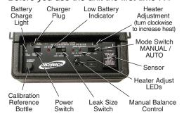
Remove the sticky-label disc from the cap of the Calibration Reference Bottle. This disc can be reused to help seal the vial when the leak detector is not in use, or it can be discarded. DO NOT attempt to unscrew the cap, you may damage the bottle! It is filled with enough refrigerant to last approximately six months.  With the Power switch in the OFF position, charge the internal battery using the furnished wall adapter. Charge time is 8–10 hours or, until the red Full Charge LED turns green.
