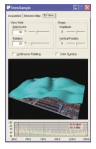
With the "3D View" function, a field intensity distribution is represented graphically. The higher the intensity, the higher the altitude. This 3D graphic rotates for easier identification.
