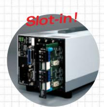
Extensible, flexible construction using the slot-in system (at the rear)
