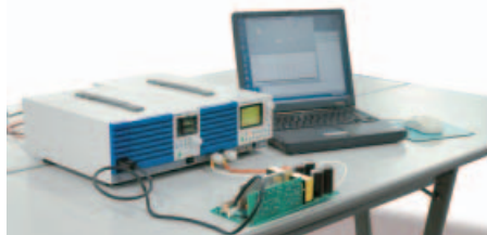
Neatly fits on your desk! (Picture) Left: PCR500M Right: Electronic Load PLZ164W
