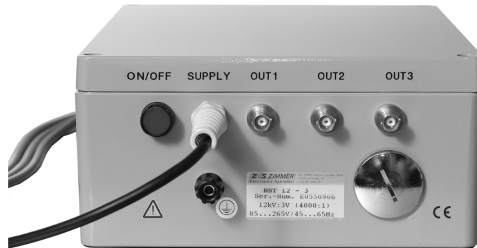
Figure 119: precision high voltage divider HST12-3
