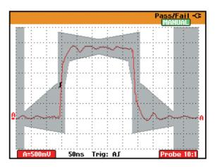
Figure 4: Pass/fail template at the ScopeMeter
